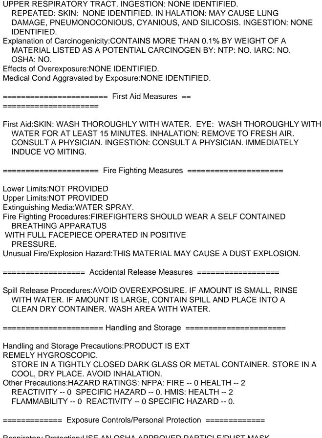
Respiratory Protection: USE AN OSHA APPROVED PARTICLE/DUST MASK. Ventilation: USE GENERAL OR LOCAL EXHAUST VENTILATIO
