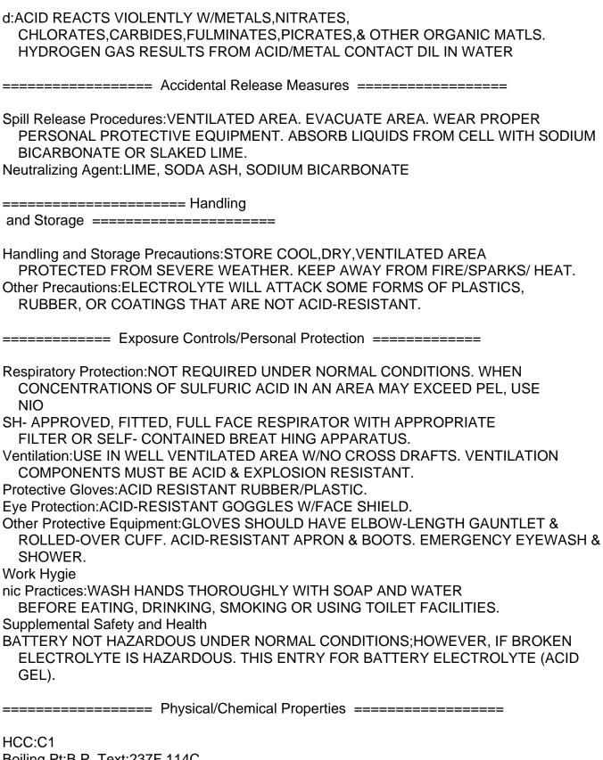
Boiling Pt:B.P. Text:237F,114C Melt/Freeze Pt:M.P/F.P Text:-94F,-70C Decomp Temp:Decomp Text:NOT GIVEN Vapor Pres:9.95 Vapor
