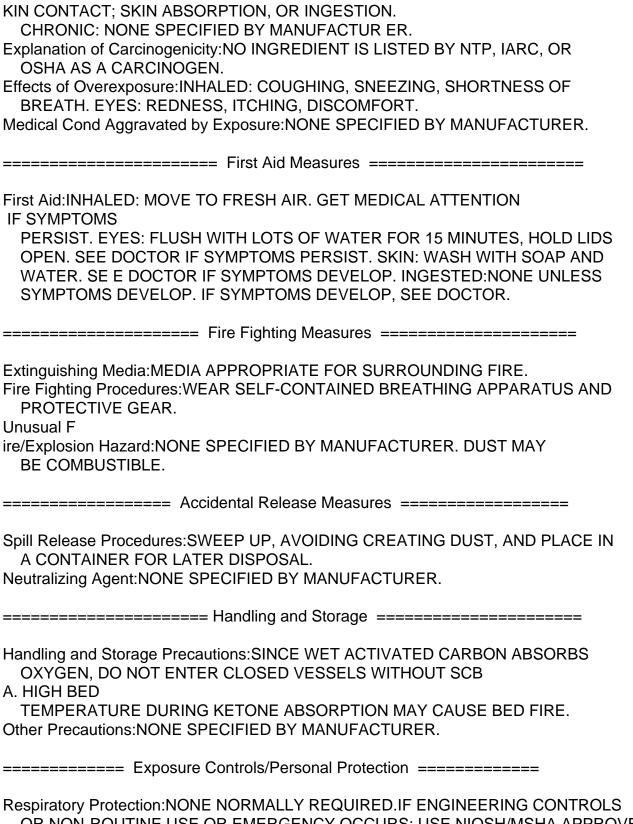
Respiratory Protection: NONE NORMALLY REQUIRED. IF ENGINEERING CONTROLS OR NON-ROUTINE USE OR EMERGENCY OCCURS; USE NIOSH/MSHA APPROVED RESPIRATOR FOR DUST OR SUPPLIED AIR RESPIRATOR OR SCBA, AS REQUIRED. USE IN ACCORDANCE WI TH 29 CFR 1910.134.
